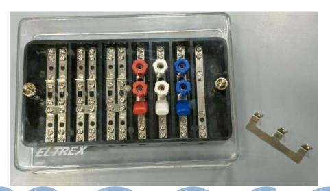
The Test Blocks offer easy access for on site testing of Ammeters, KWH Meters, Maximum Demand Indicators, Trivector Meters, Relays and Instrument Transformers without disconnecting from load and avoid C.T. open circuit problems. Connections for testing can be easily made. The Test Block therefore becomes an important element of the Metering Solution.
