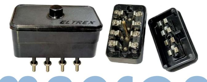
These 4 Way Test Blocks are used for mounting on switchboard panels for use with proper test equipment's to facilitate the testing of AC instruments, meters and relays.
